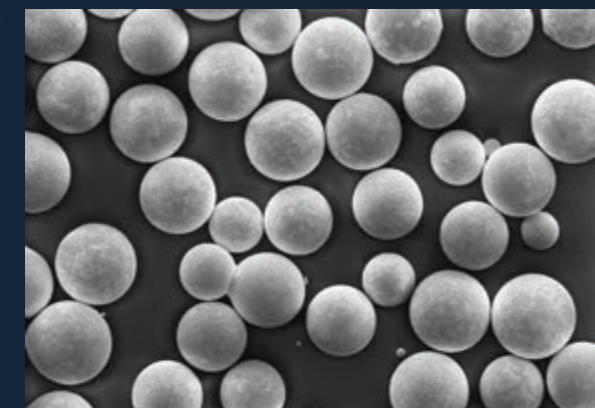
Unsieved, raw ATO LAB powder, note the uniform size and spherical shape of the particles
